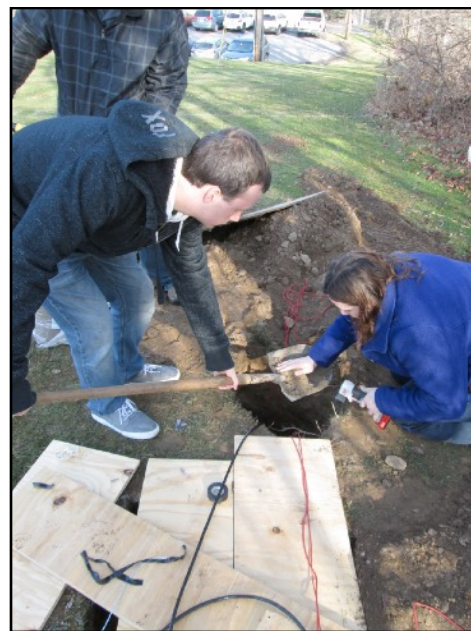
Left image - Colgate's new seismic stations in the Adirondack Mountains (red squares) in relation to existing stations. Large earthquakes from the past shown by white circles. Right image - Sean Corrigan (Astrogeophysics '18) helps to carefully bury the sensitive seismometer at Colgate's on-campus seismic station in December 2015.
